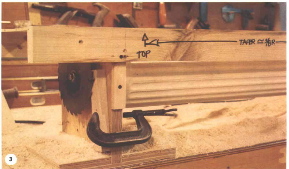
Jigging and assembly. The column shafts were turned and fluted with the use of a shop-built, benchtop router jig. The core of the jig was a \frac{1}{2} -in. galvanized iron pipe that suspended the shafts between a pair of plywood turning centers. The hollow shafts were plugged at both ends with a combination plywood cap and wooden clamp that accommodated the axle and clamped the shafts to it (photo 1). For turning, the axle was fitted with a 12-in. pulley belted to an adjacent shop lathe (photo 2). At the opposite end, a 24-tooth circular-saw blade (mounted backwards for safety) served as an indexing head (photo 3).
